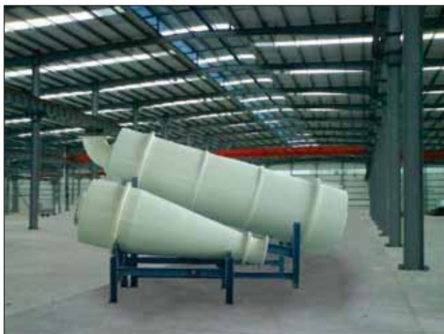
Fig 2: Three-Product Dense Medium Vessel
